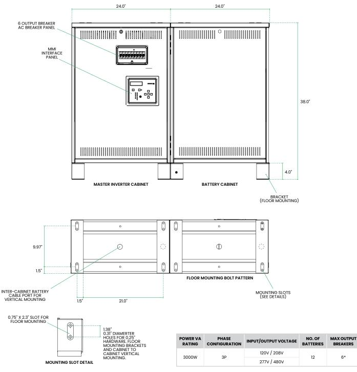
NOTE: Breakers must be a multiple of three to ensure even load distribution.
