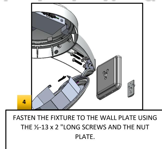
FASTEN THE FIXTURE TO THE WALL PLATE USING
