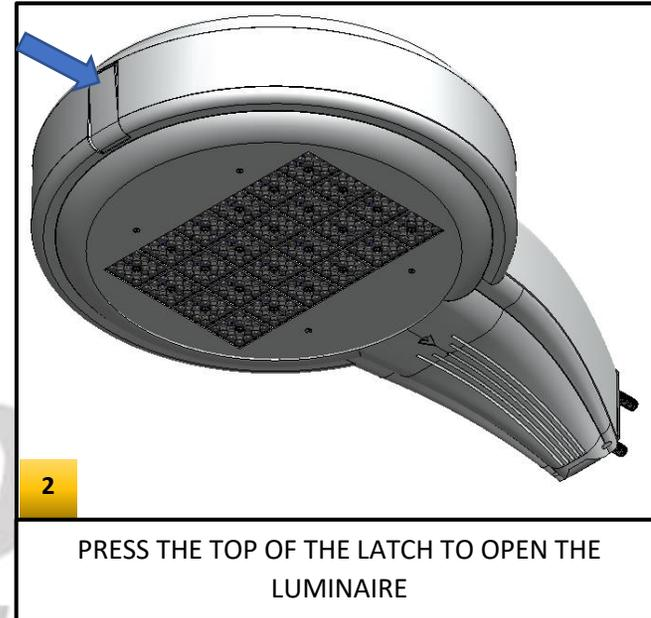
PRESS THE TOP OF THE LATCH TO OPEN THE
