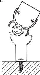
**2c** When one corner is inside the clip, turn fixture to "roll" the rest into the clip.
