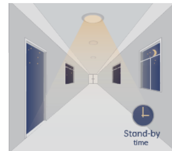
After hold time, sensor dims light to stand-by dimming level for stand-by time.
