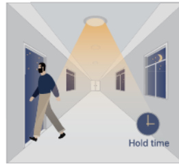
After there's no motion detected, the sensor keeps light ON brightness setting for hold time.
